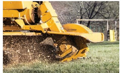
**MINIMIZED RECIRCULATION.** The wheel design and placement of the teeth allows for material to flow efficiently past the wheel after being cut, minimizing the recirculation of material.
