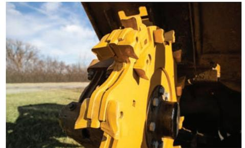
**DOUBLE-SIDED TOOTH.** The two cutting edges on the Vermeer cutting system tooth provide the operator an advantage by giving the edges two times the wear.
