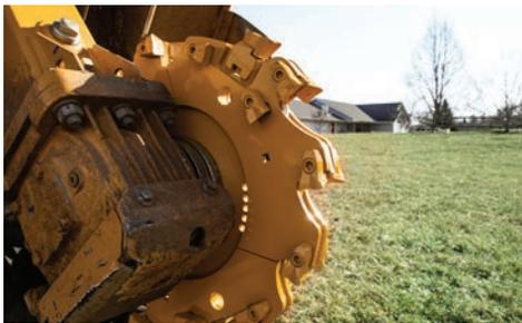
**CENTER CORE PROTECTION.** Wear plates on each side help protect the machined center core. They are made of high abrasion-resistant steel and can be replaced at a cost lower than having to buy an entirely new wheel.
