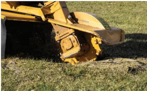
**EASE OF MAINTENANCE.** This wheel offers convenient features such as the single bolt for all teeth, which only requires two tooth part numbers and no other wear parts to maintain. Once torqued, the bolts remain tight until the teeth are removed or flipped.
